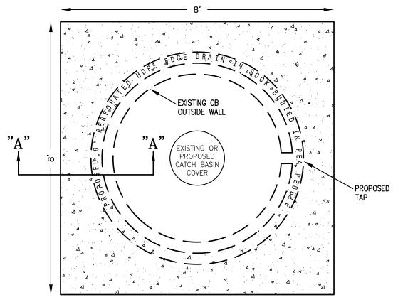
8" CONCRETE COLLAR & 6" EDGE DRAIN PLAN DETAIL & SECTION (NOTE: ADJUST AS NECESSARY AROUND CATCH BASINS IN GUTTERS OR NEXT TO WALKS)
